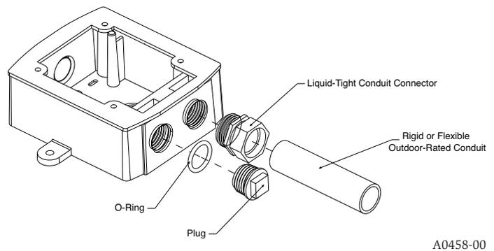
Remember to plug any unused conduit openings with the conduit plugs provided (see How to Install Conduit Plugs).
