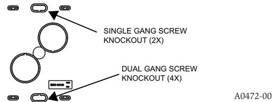
**FIGURE 4. SCREW KNOCKOUT REMOVAL WITH SCREWDRIVER:**
