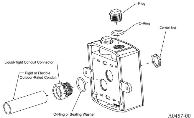
**FIGURE 6: INSTALL IN TOP THREADED OPENINGS**
